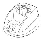
**CHARGE** and **BATT CHARGE** LEDs indicate battery charging status. The LEDs flash red when charging, and are steady red when the battery is charged.
